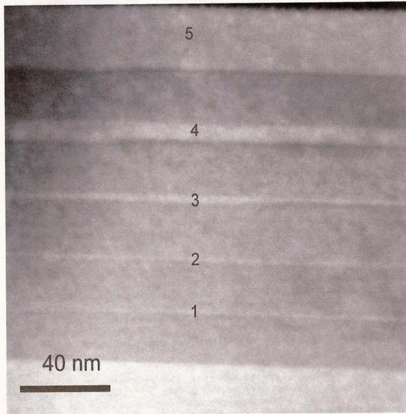
Figure 1. Transmission electron microscopy (ADF-STEM) cross sectional image of AlGaN/GaN multi quantum well structure grown by novel HVPE method at TDI, Inc. (courtesy Prof. Subhash Mahajan, Arizona State University). Five GaN layers having thickness of about 2 nm, 3 nm, 4 nm, 8 nm, and 25 nm are sandwiched between AlGaN barrier layers having thickness of 20 nm.
