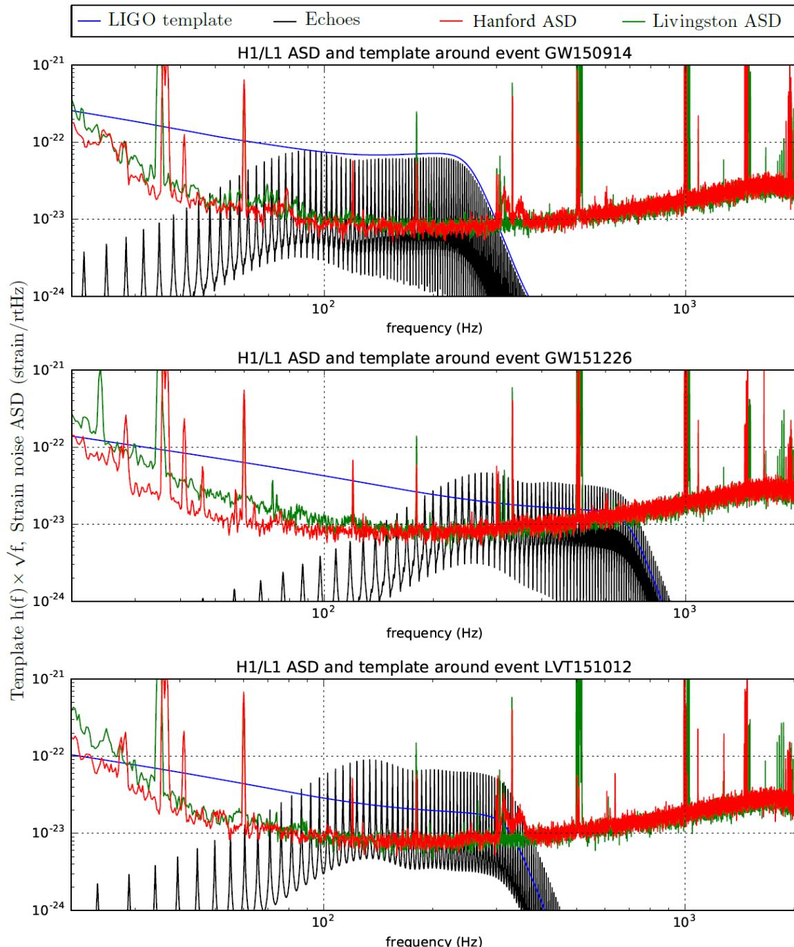
Best fit templates for LIGO main events and echoes (using the joint best fit), in Fourier space. The amplitude spectral distribution (ASD) for each detector is shown for comparison.
